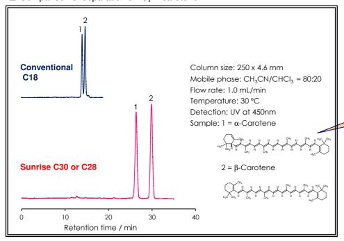
The mobile phase including chloroform makes alkyl chains brash up because chloroform can enter among alkyl chains. Consequently retention times of C30 or C28 became 2 times longer than C18.
