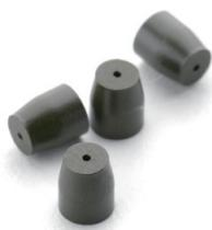
The graphite vespel ferrule is suitable for GC/MS with mechanical strength and the graphite ferrule for general GC. Both types have excellent stability when the temperature increases and chemical resistance. Blister package is adapted for graphite vespel ferrule.
