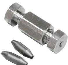
This is the micro union with zero dead volume. Polyimide resin is adapted for the ferrule for better heat resistance and chemical resistance.
