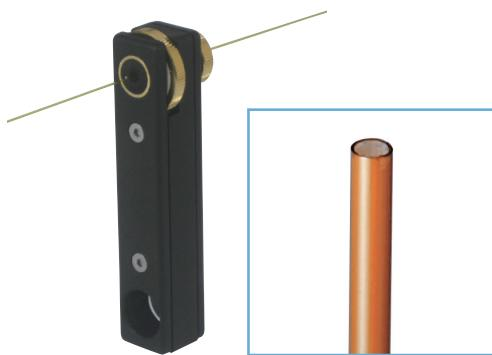
A diamond blade finely cuts the silica capillary tube vertically. The built-in magnifier is to check how the tube is cut, and the diamond blades can be replaced.
