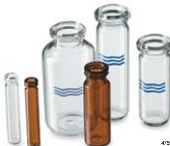
Serum bottles are made of borosilicate glass that has a higher coefficient of expansion than autosampler vials. They have less resistance to sudden temperature changes.
