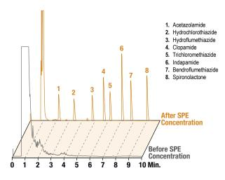
Column: Alltima™ C18, 3µm, 100 x 4.6mm HPLC Column (Part No. 81382)
