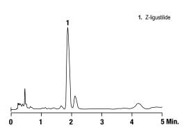
Column: Alltima™ C18, 3µm 53 x 7mm Rocket™ HPLC Column (Part No. 50605)
