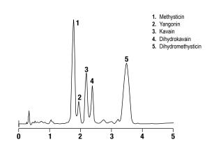
Column: Alltima™ C18, 3µm, 53 x 7mm Rocket™ HPLC Column (Part No. 50605)
