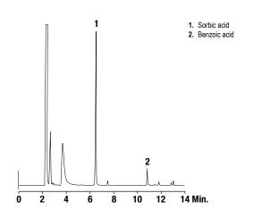
**Column:** Heliflex® AT™ AquaWax-DA, 30m x 0.25μm Capillary GC Column
