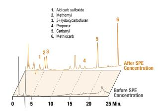
Column: Platinum™ EPS C18, 5µm, 250 x 4.6mm HPLC Column (Part No. 32246)
