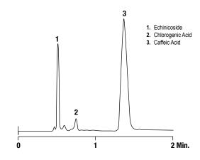
Column: Alltima™ C18, 3µm 53 x 7mm Rocket™ HPLC Column, (Part No. 50605)
