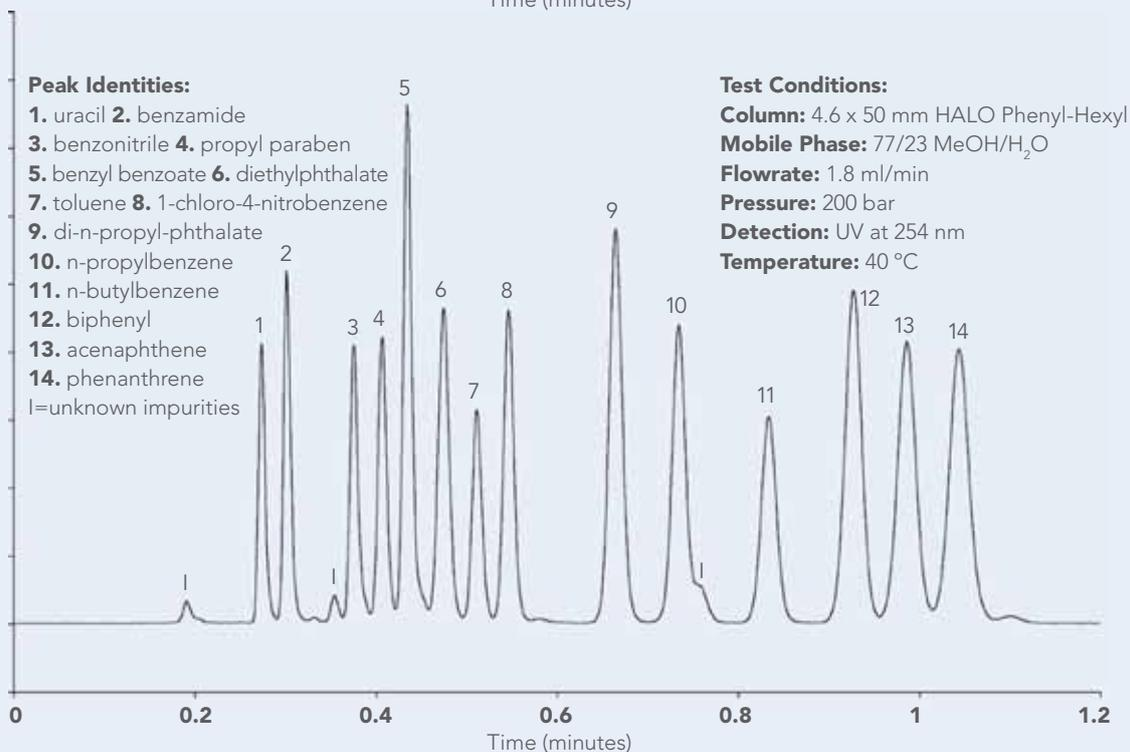
These two chromatograms illustrate how HALO Phenyl-Hexyl columns can provide separation of complex mixtures in a little over a minute.
