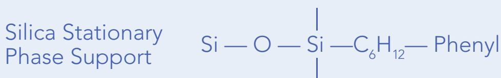
A phenyl group is bonded to the silica surface via a hexyl chain.
