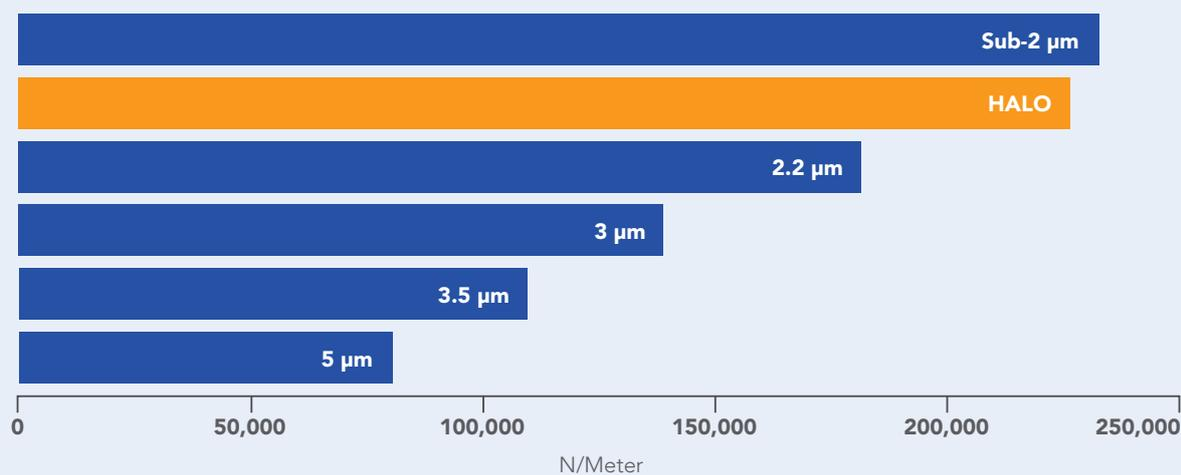
HALO columns deliver over 90% more separating power (theoretical plates) than columns of the same length packed with 3.5  $\mu\text{m}$  particles and almost three times the separating power of columns packed with 5  $\mu\text{m}$  particles.
