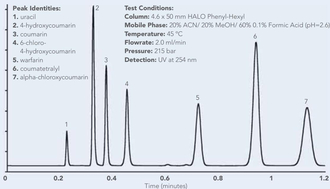
Six anticoagulants are well separated on a HALO Phenyl-Hexyl column in less than 72 seconds.
