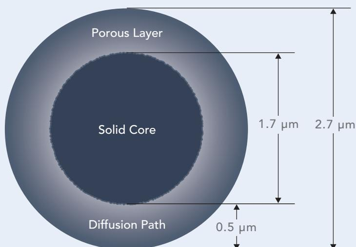
Fused-Core particle technology was developed by Jack Kirkland to produce UHPLC columns that could be effectively used with either UHPLC or conventional HPLC equipment. As the name implies, Fused-Core particles are manufactured by fusing a porous silica layer onto a solid silica particle.
