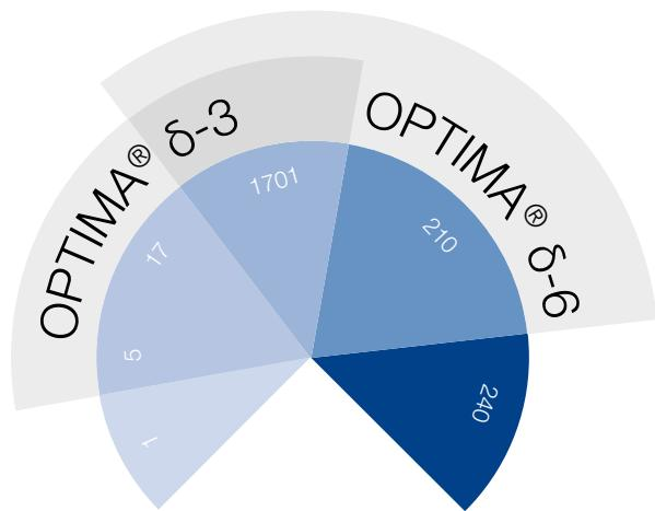
All stationary GC phases can be classified by their polarities. While the selectivity of common GC phases is generally determined by permanent dipole-dipole interactions, OPTIMA® δ-3 and OPTIMA® δ-6 show an additional feature. Large, polarizable groups in the polymer chain of the stationary phase enable the analyte to induce a further dipole moment that increases
