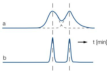
R: resolution: a measure for the quality of a separation, taking ( $w_{1/2}$ ) into account according to:
