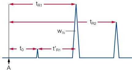
A: starting point of a chromatogram = time of injection of a dissolved solute
