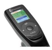
eVol® features a familiar Touch Wheel user interface and a full-color screen. The clever menu allows all the functions to
